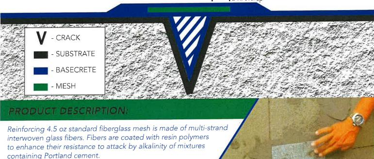
Basecrete Fibermesh is used to reinforce & strengthen Basecrete in applications with a high level of stress and/or applications that are expected to have a high degree of movement in them.
